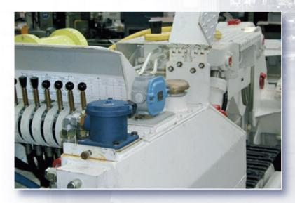
Level and temperature switch iTNA01 used for monitoring the hydraulic fluid in a loader car
