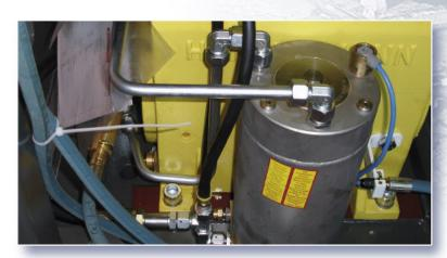
Monitoring the temperature of the lubricating oil in a pump unit
