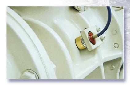
Monitoring the surface temperature of a screw-type compressor
