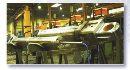
Installing the reed contact rod into a ranging arm lifting cylinder
