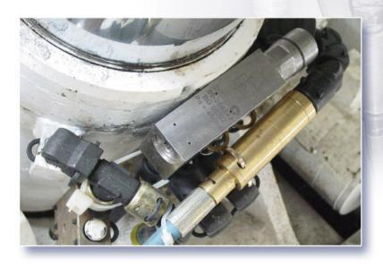
Monitoring the leg pressure in a shield support underground
