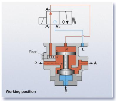
For the "negative" design the pilot valve in rest position is opened and closed in working position.
